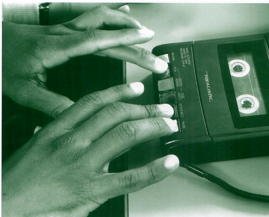
Operating a tape recorder with tactile labels on the controls
